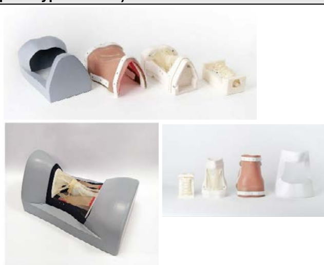
Figure 1 - V.1 Prototype of the Physical Anatomic Phantom - Chassis and internal structures.
