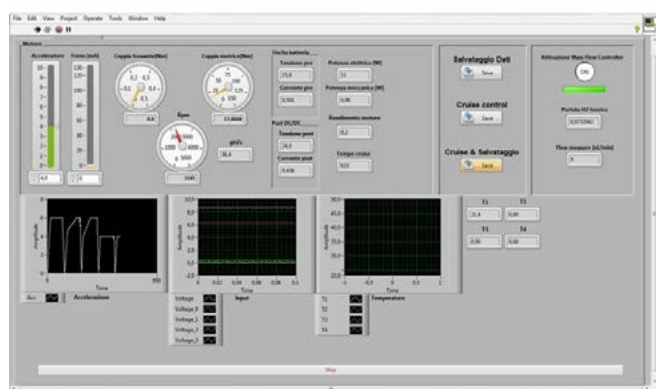
Figure 2 - Control system - LabVIEW code
