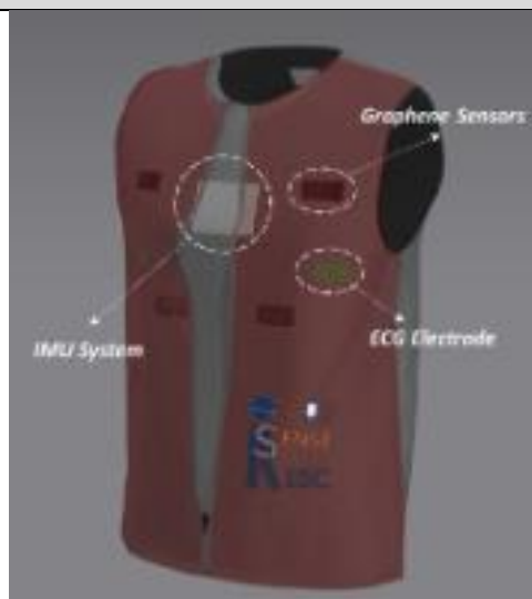
Figure 2 -wearable t-shirt with Bluetooth systems for physiological monitoring
